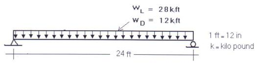
5. Design a cover-plate beam no greater than 16 in. in depth to support a dead service uniform load  $w_D$  of 4 k/ft (not including the beam weight) and a live service load  $w_L$  of 6 k/ft for a 24 ft simple span. Use A572 steel with  $F_y = 50$  ksi with full lateral bracing of the compression flange. Use a W14 beam plus cover plates. .(13 points)
