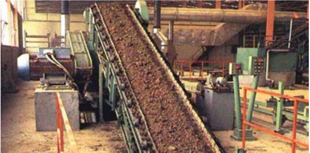
Material being moved via-belt conveyor.
