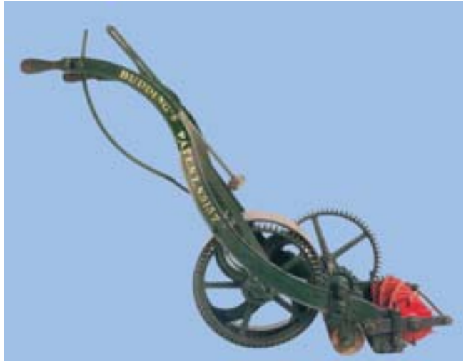
Lawn-mover is a combination of kinematic links.
