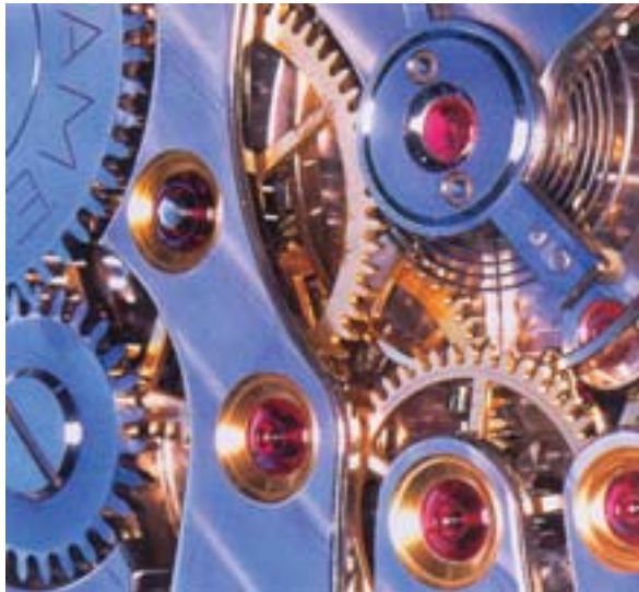
Gear trains inside a mechanical watch
