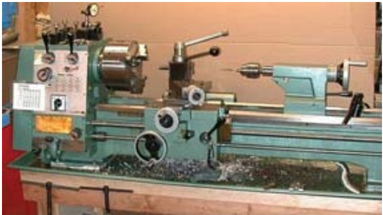
A lathe is a machine for shaping a piece of metal, by rotating it rapidly along its axis while pressing against a fixed cutting or abrading tool.
