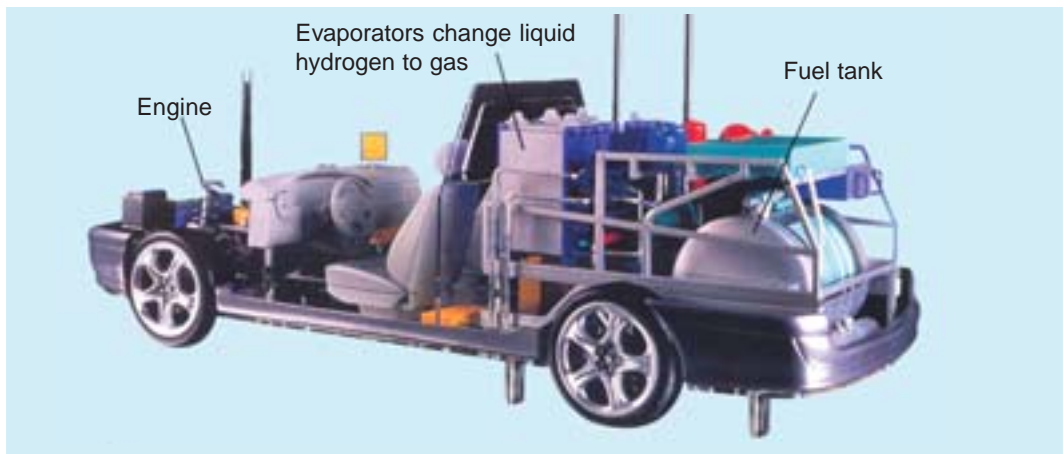
This experimental car burns hydrogen fuel in an ordinary piston engine. Its exhaust gases cause no pollution, because they contain only water vapour.
