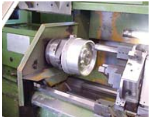
A pulley is being processed at a turning centre.
