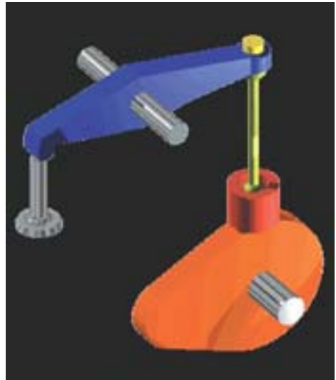
A rocker using a cam.
