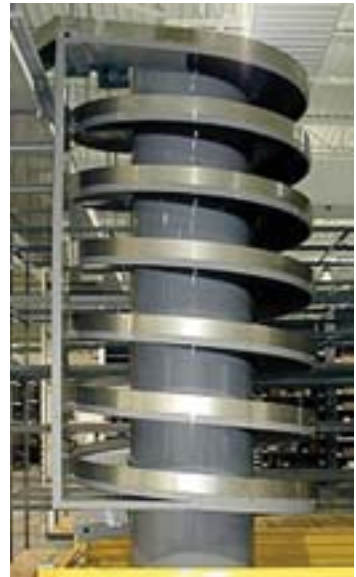
A spiral elevator conveyor for material handling.
